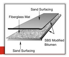
Meets or exceeds performance requirements of ASTM D 6163, Type I, Grade S
