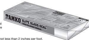
USES: For application to roof decks with inclines of not less than 2 inches per foot. For slopes between 2 inches and 4 inches per foot, refer to application instructions for low slope.
